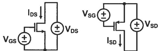
$$\text{Saturation: NMOS } I_{DS} = \frac{1}{2} K_P N \frac{W}{L} (V_{GS} - V_{TN})^2$$
