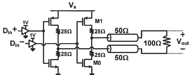
a) Output voltage swing =  $1 V_{ppd}$
