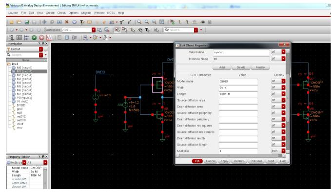
When finished, your schematic should resemble shown Figure to measure FO4 Delay. Select Design  $\rightarrow$  Check and Save to save your schematic and make sure that there are no errors or warnings.
