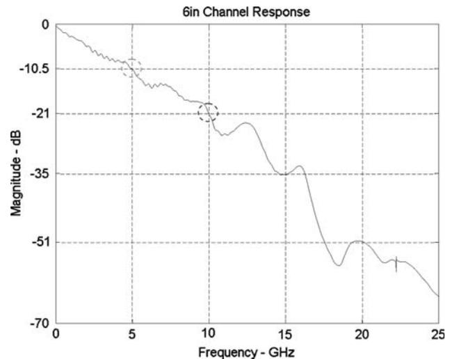
**Fig. 5** Target clock channel frequency response for a six inch channel across an FR4-based printed circuit board
