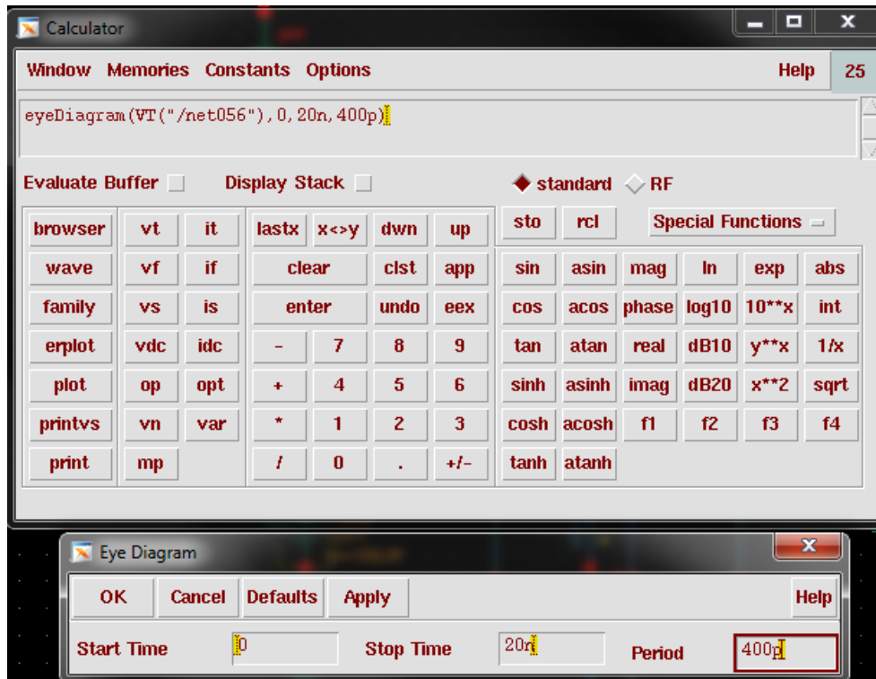
Figure 18 How to Plot Eye Diagram in Cadence Using Calculator
