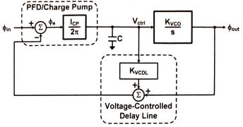
a) Find the expressions for the open loop gain, LG(s), the phase error transfer function, E(s)=\$\phi\_e(s)\$/\$\phi\_in(s), and the closed-loop transfer function H(s)=\$\phi\_out(s)\$/\$\phi\_in(s). (25 points)
