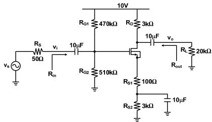
5. **(20 points – 10pts calc., 10pts Multisim)** Common Drain Amplifier. Repeat parts a) and b) from Problem 4 for the common drain amplifier.
