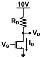
What is the  $maximum R_D$  such that the transistor remains in the saturation region with
