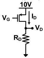
What is the  $maximum R_D$  such that the transistor remains in the saturation region with
