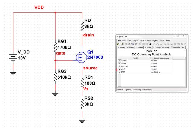
4. Common Source Amplifier  $A_{V} = -\frac{g_{m}(R_{o}||R_{L})}{|+g_{m}R_{s}|} = -\frac{(|4.3^{ma}/_{v})(3kn|/20kn)}{|+(|4.3^{ma}/_{v})(100k)}$  $Av = -15.4 \ v = 23.7 dB$ Rin = Ra = 470KN//SIOKN = 245KN R:n = 245KR = 108dBR Rout = Ro = 3kl = 69,5dBR  $G_{v} = \frac{R_{in}}{R_{in} + R_{vs}} A_{v} = \frac{245 k L}{245 k L + 50} (-15.4)$  $G_{v} = -15.4 V_{v} = 23.7 JB$
