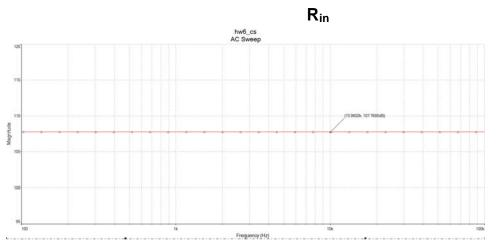
The simulated  $R_{in}$  value of 108dB $\Omega$  matches the hand calculation of 108dB $\Omega$ .
