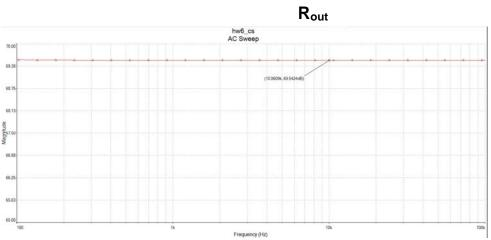
The simulated R<sub>out</sub> value of 69.5dB $\Omega$  closely matches the hand calculation of 69.5dB $\Omega$ .
