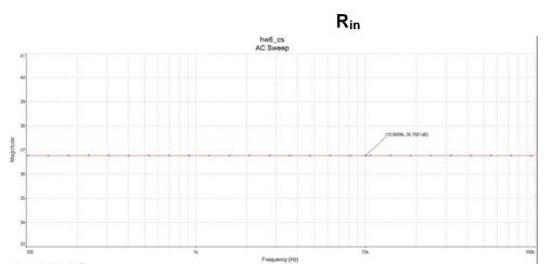
The simulated  $R_{in}$  value of 36.8dB $\Omega$  matches the hand calculation of 36.7dB $\Omega$ .
