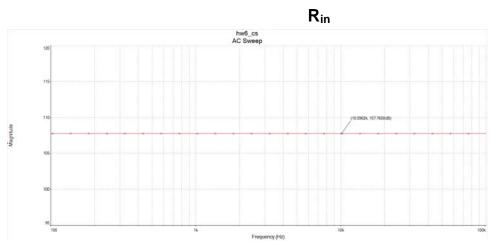
The simulated  $R_{in}$  value of 108dB $\Omega$  matches the hand calculation of 108dB $\Omega$ .
