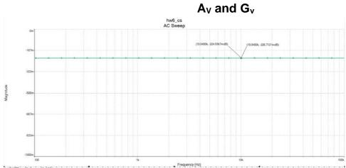
The simulated value of -0.22dB and -0.23dB closely matches the hand calculation of -0.22dB for both  $A_v$  and  $G_v$ , respectively.
