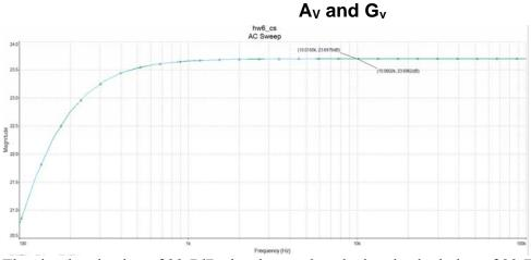
The simulated value of 23.7dB closely matches the hand calculation of 23.7dB for both  $A_v$  and  $G_v$ .
