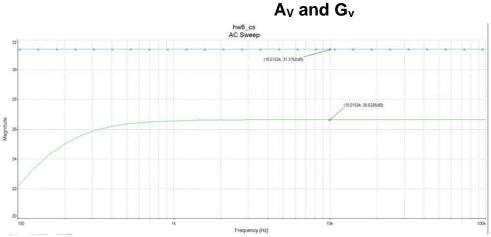
The simulated  $A_v$  value of 31.4dB matches closely the hand calculation of 31.4dB. The simulated  $G_v$  value of 26.6dB closely matches the hand calculation of 26.7dB.
