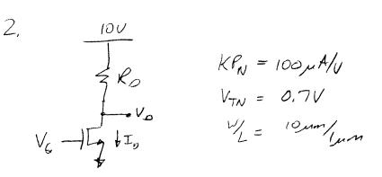
Max to for saturation =  $\frac{10V - Vossat}{IosAT}$
