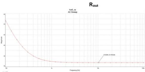
The simulated R<sub>out</sub> value of 36.8dB $\Omega$  closely matches the hand calculation of 36.7dB $\Omega$ .
