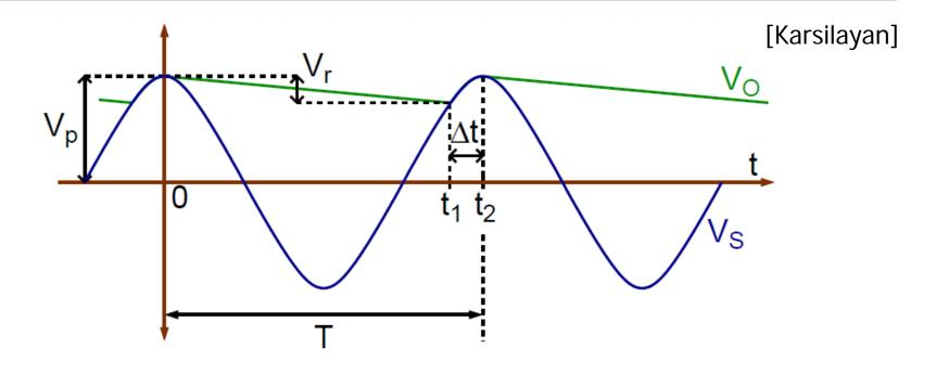
$$\begin{split} & V_p \cos(\omega \Delta t) = V_p - V_r \\ & \omega \Delta t \text{ is small } \Rightarrow & \cos(\omega \Delta t) \approx 1 - \frac{1}{2} (\omega \Delta t)^2 \end{split}$$
