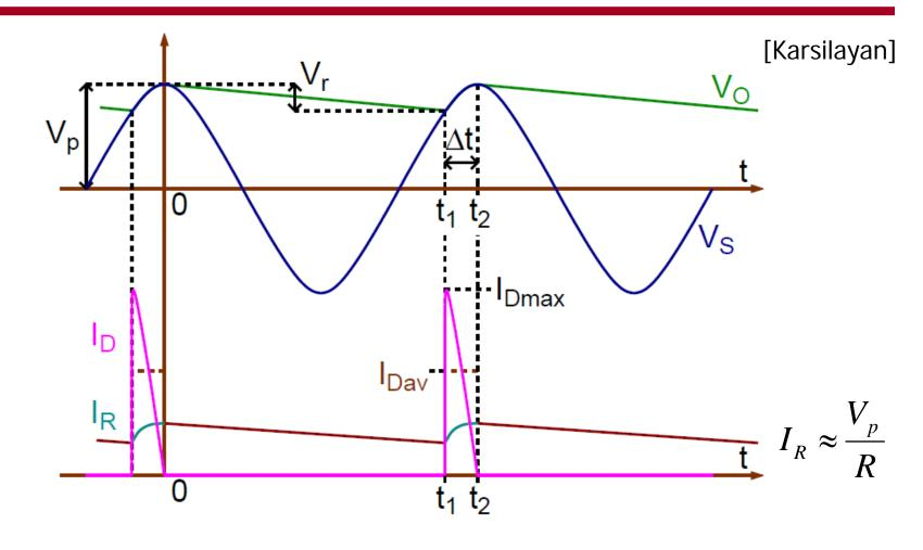
During conduction  $(t_1-t_2)$ :  $Q_{supplied} = Q_{lost}$   $I_{Cav}\Delta t = CV_r$
