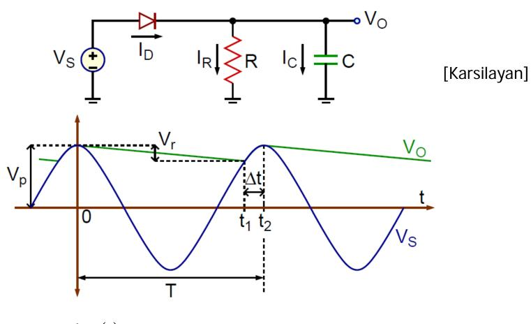
$$V_{o}(t) = \begin{cases} V_{s}(t) - 0.7V, t_{1} < t < t_{2} \\ V_{p}e^{-\frac{t}{RC}}, 0 < t < t_{1} \end{cases} \Rightarrow V_{o}(t_{1}) = V_{p}e^{-\frac{t_{1}}{RC}}$$
