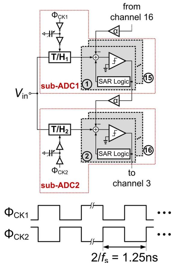
Fig. 8. Block diagram of the 16-way time-interleaved SAR ADC with embedded one-tap DFE.
