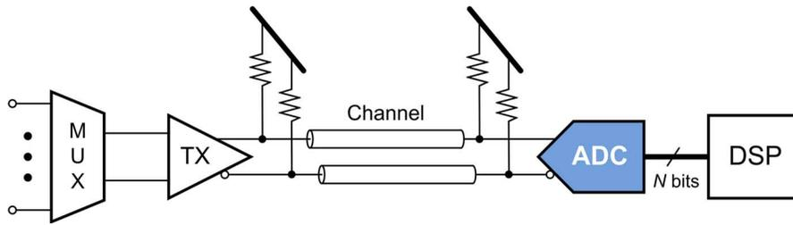
Fig. 1. High-speed link with an ADC-based receiver.
