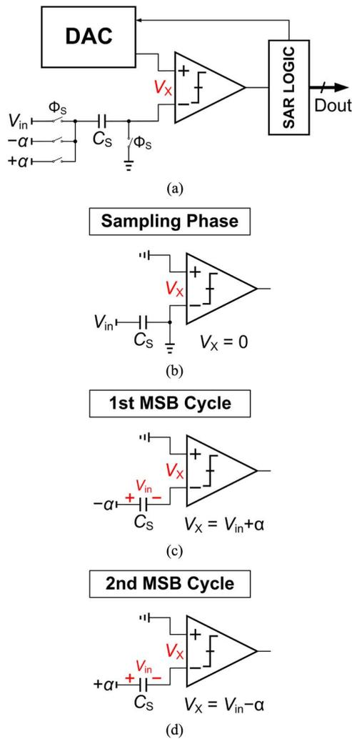
Fig. 7. SAR ADC with embedded one-tap DFE. (a) Simplified block diagram, operation during the (b) sampling phase, (c) first MSB evaluation, and (d) second MSB evaluation.
