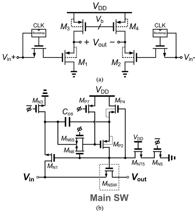
Fig. 11. Front-end T/H. (a) Schematic. (b) Bootstrapped switch structure.
