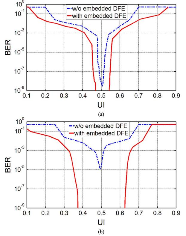
Fig. 20. Measured bathtub curves for the (a) 30-in smooth and (b) 28-in notch FR4 channels shown in Fig. 3, with and without one-tap embedded DFE for a  $2^{10} - 1$  PRBS input with 300- $mV_{pp}$  TX swing and no TX equalization.
