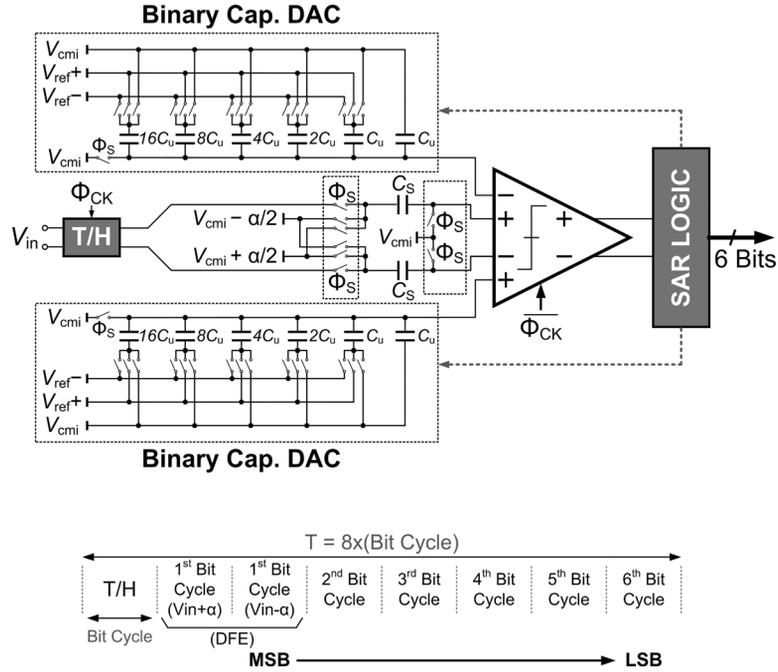
Fig. 9. Unit SAR ADC schematic with redundant cycle embedded one-tap DFE.
