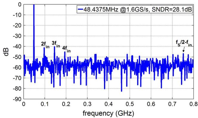
Fig. 15. The 1.6-GS/s ADC normalized output spectrum for  $f_{in} = 48.437$  MHz.
