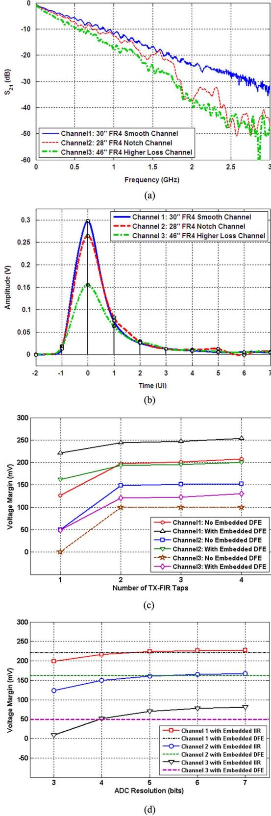
Fig. 3. (a) Magnitude and (b) 1.6-Gb/s pulse responses of three FR4 channels. (c) Impact of including one tap of embedded DFE equalization for different levels of TX-FIR equalization. (d) Impact of ADC resolution with embedded DFE and embedded IIR equalization with no TX FIR equalization over three FR4 channels.
