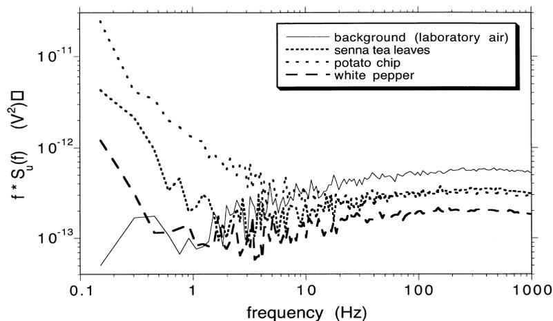
Fig. 2. Demonstration of the usefulness of the new sensor principle. The voltage noise spectrum  $S_u(f)$  of the sensor (proportional to the resistance noise spectrum) was measured at a current of  $125 \mu\text{A}$  during exposition of the sensor to different types of natural odors. The differences between the shape of the spectra should be noticed.
