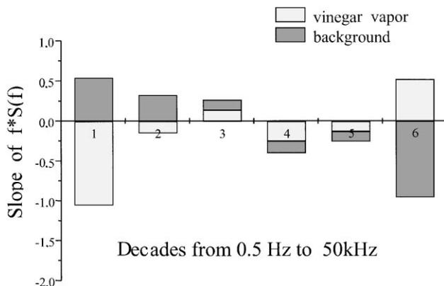
Fig. 3. Example of a way of pattern generation from the noise spectrum. The pattern was generated by the mean value of the slope in the log–log plot of the  $f^*S(f)$  function in the different frequency decades. The background data were obtained in the laboratory air.
