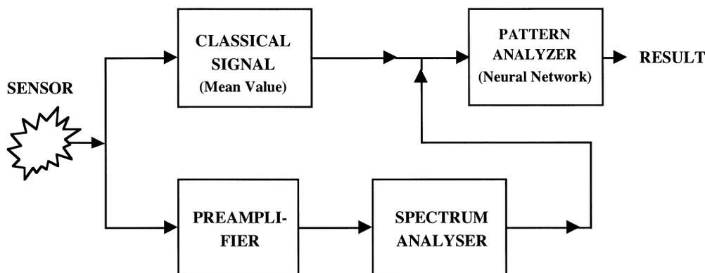
Fig. 1. Possible realization of the electronic nose or tongue principle [13]. The mean resistance and the resistance noise spectrum are measured. The spectrum is analyzed by a pattern recognition technique.
