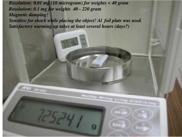
**Figure 3.** The scale, the humidity and temperature gauge, and a 2 GB flash drive. For more details see the text in the figure. At the experiments reported here the flash was placed on the scale together with a handmade Al foil plate which helped to reduce the shocking of the scale thus the induced offset was negligible.
