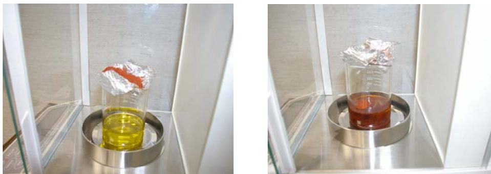
**Figure 11.** "Writing information" into a media in a natural way: dissolving chilli pepper in olive oil. Left figure: initial total mass measurement of the  $40 \text{ cm}^3$  extra virgin (cold press) olive oil in the glass, and 4.3 gram chilli powder above it in the Al foil plate. Right figure: total mass measurements during "writing". See Figure 12.
