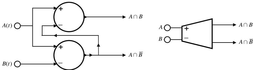
Fig. 3. Left: The neural circuit of the *orthon* [5]. Right: Its symbol.
