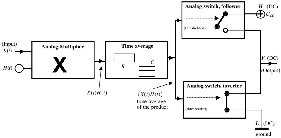
Fig. 5. The FOLLOWER gate of the classical (“slow”) noise-based logic used as interface toward regular (DC) digital circuitry. The time-averaging procedure, which is essential for the input correlator of the “slow” logic, together with the threshold of the output switches, removes the (fast) errors [1].
